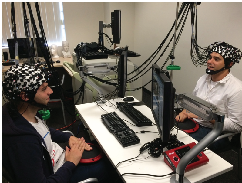
Fig. 2. Experimental set-up for two interacting partners in the drumming condition. The talking communication condition was identical, but without the drum apparatus.
